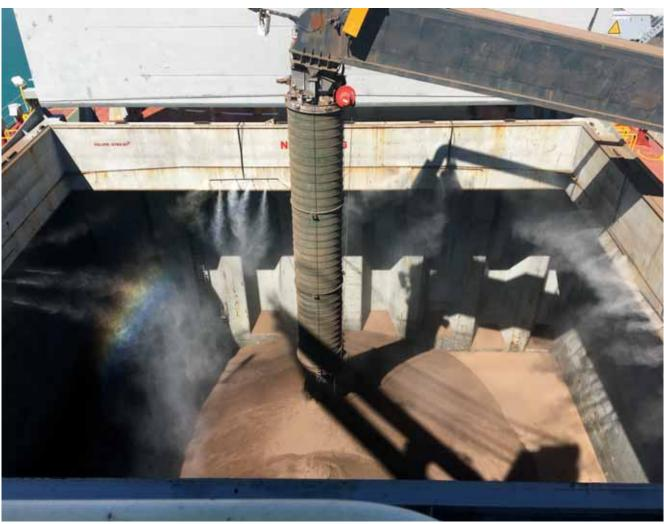
Blue Water Misting (BWM) was selected by an Australian client to supply its Dry Fog system for use in shiploading operations. The client is located close to a residential area, so the need for dust-free loading systems is paramount.
